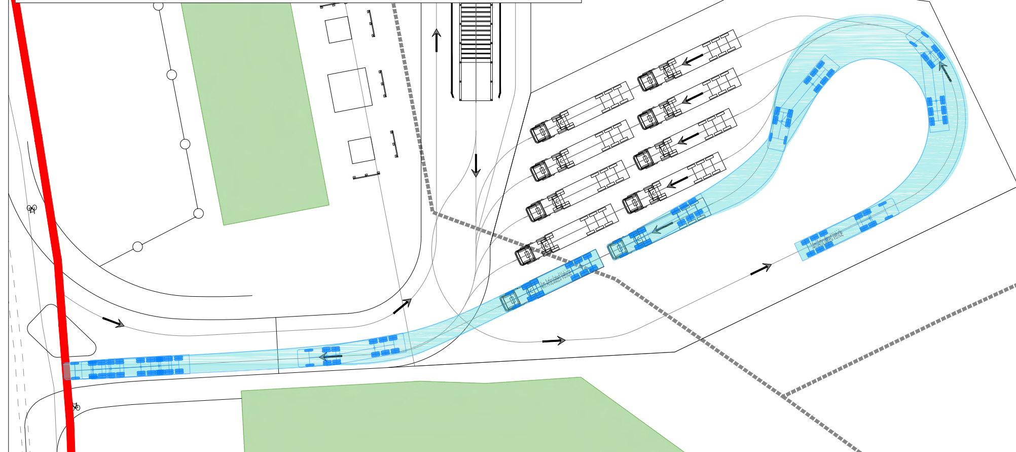
14m ARTICULATED VEHICLE ROUTING THROUGH WAITING AREA
