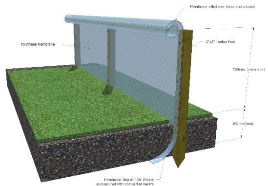
Figure 4: example diagram of non-permanent 'drift' herptile fencing specifications and installation method
